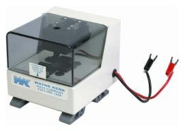
1009 Fixture enables 50 A to be applied to an SMD inductor
